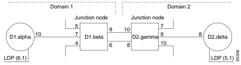
The dspnwrt command must be entered at node D1.alpha or D2.delta (the end points of the connection).
