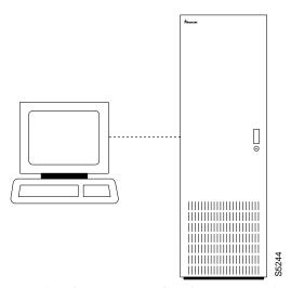
A workstation or a PC can function as a control terminal for an IPX, IGX, or BPX through an RS-232 link or over an Ethernet TCP/IP LAN. All command input takes place at the terminal, and all displays appear on the terminal screen. Through displays that show status, alarm, or statistics, the terminal constantly provides a view of an individual node, a trunk, a connection, or the whole network.
