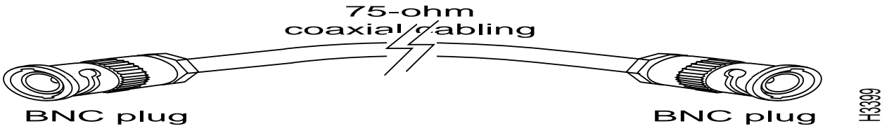
Figure 3-16 75-ohm Coaxial Data Cable
