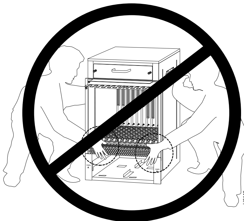
Figure 3-2 Incorrect Way to Lift the Cisco 7513
