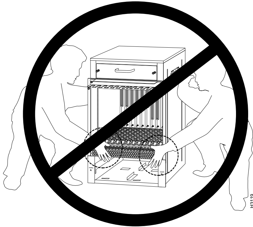
Figure 2 Incorrect Way to Lift the Cisco 7513
