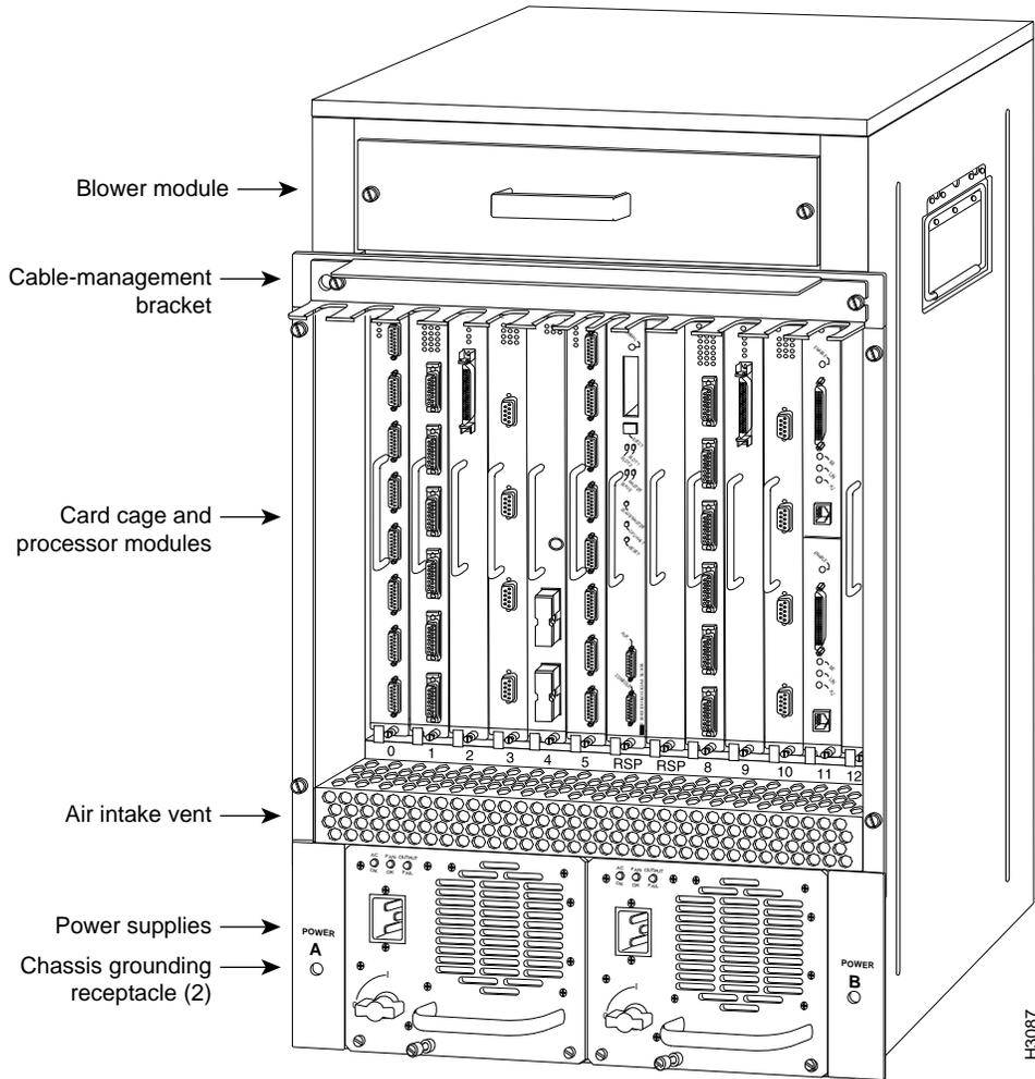
The blower module assembly comprises the blower, a printed circuit board (control board) mounted on a metal plate, three front panel LEDs, a power connector, and a metal case with a handle. A view of the end of the blower module (opposite the end with the handle) is shown in Figure 2.
