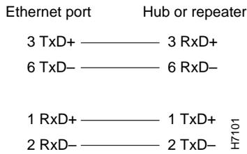
**Figure 7 Crossover Cable Pinout, 8E RJ-45 Connections Between Hubs and Repeaters**
