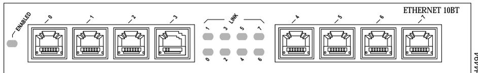
The 8E port adapter can be installed on the VIP2 in port adapter slot 0 and port adapter slot 1, or in the Cisco 7200 series routers in any of the chassis' port adapter slots: 1 through 6 for the Cisco 7206. Port adapters have a handle attached, but this handle is occasionally not shown to allow a full view of detail on the port adapter's faceplate.
