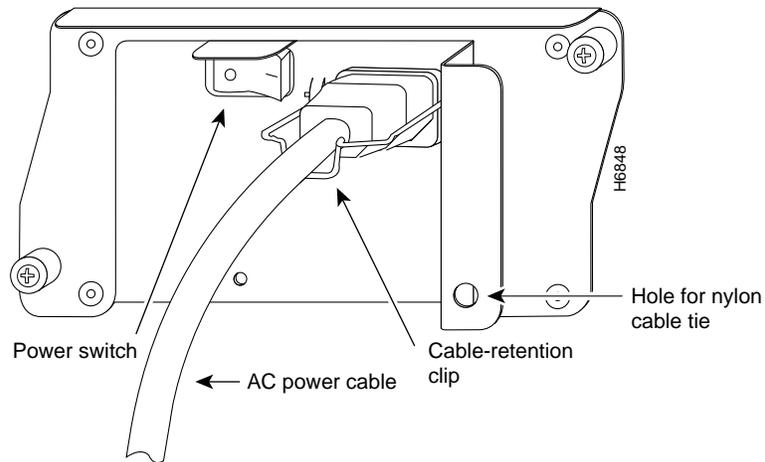
**Step 4** Plug the AC power supply cable into the AC power source.
