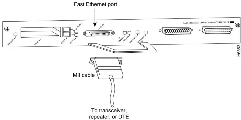
Depending on the type of media you use between the MII connection and your switch or hub, the network side of your 100BASE-T transceiver should be appropriately equipped with ST-type connectors (for optical fiber), BNC connectors, and so forth.
