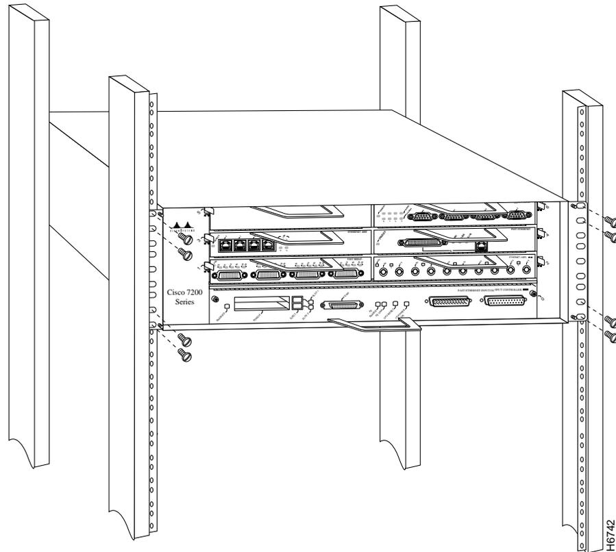
We recommend that you allow at least one or two inches of vertical clearance between the router and any equipment directly above and below it.
