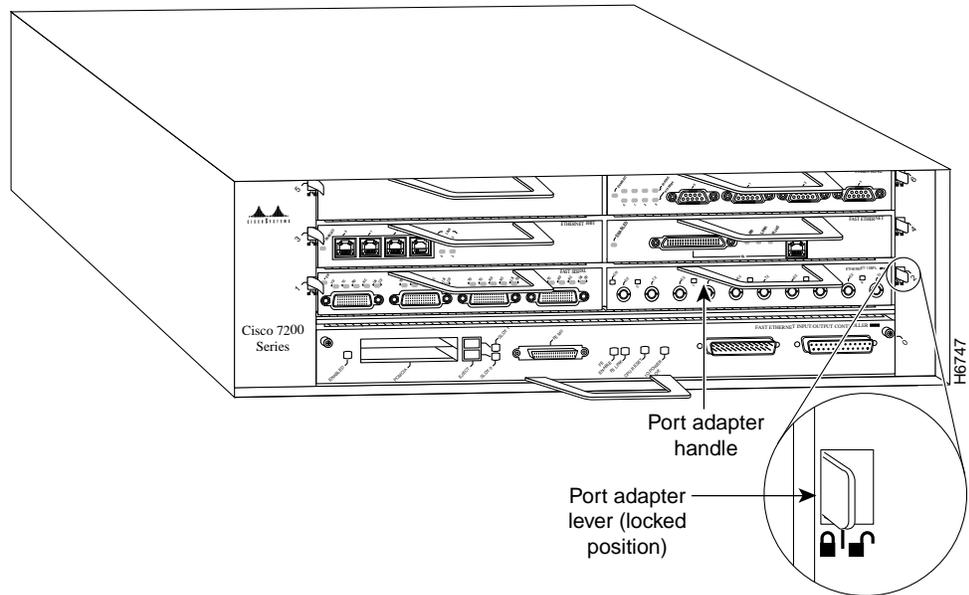
This completes the procedure for installing a port adapter in the Cisco 7206 router.
