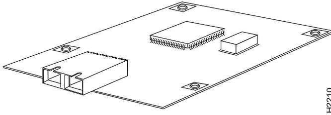
The SONET multimode SC-duplex connector is shipped with a dust plug. (See Figure 15.) Remove the plug by pulling on the plug as you squeeze the sides.
