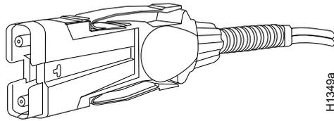
For SONET/SDH multimode connections, use one multimode duplex SC connector (see Figure 9) or two single SC connectors. (See Figure 10.)
