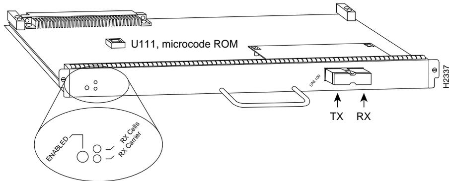
The ATM network interface for a Cisco 7000 series router resides on a modular interface processor, the AIP, which provides a direct connection between the high-speed Cisco Extended Bus (CxBus) and the external networks. The physical layer interface module (PLIM) on the AIP determines the type of ATM connection. There are no restrictions on slot locations or sequence; you can install an AIP in any available interface processor slot.
