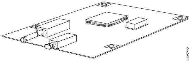
For E3 and DS3 connections, connect the coaxial cable to the BNC connector on the E3 or DS3 PLIM. (See Figure 17.)
