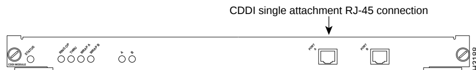
Figure 4-9 Single Attachment Station, CDDI Network Connections
