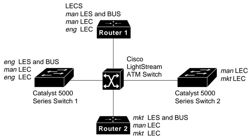
In this example, Router 1 has the following LANE components:
