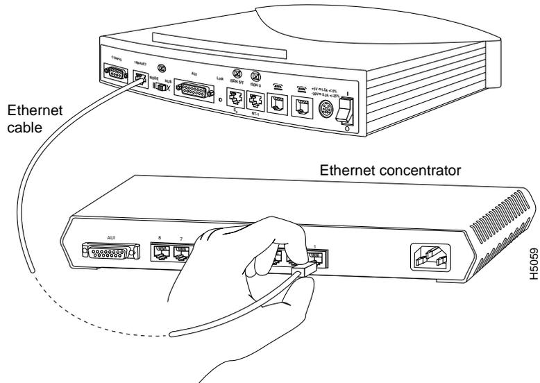
Figure 3-3 10BaseT Cable to PC NIC Connection (Cisco 766 Shown)
