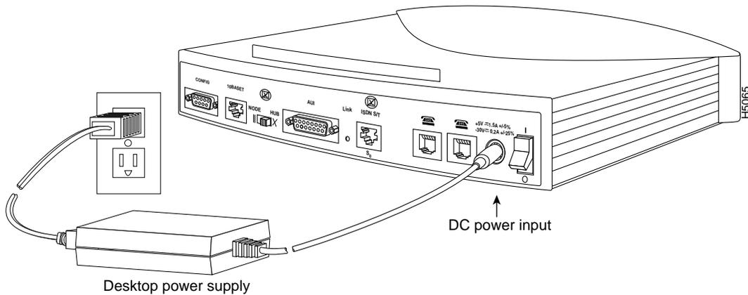
**Step 4** The router can now be powered on. Turn ON the Cisco 750 series routers with the switch labeled ON/OFF on the rear panel of the router. Turn ON the Cisco 760 series routers with the switch labeled | / 0 on the rear panel of the router.
