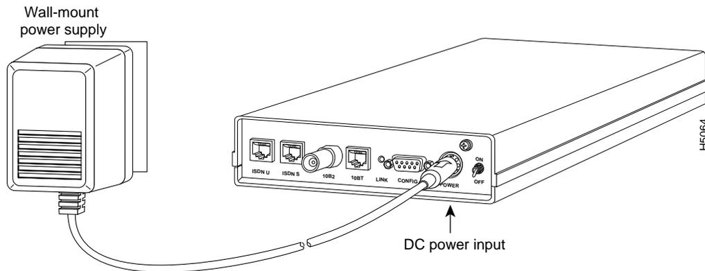
**Step 3** Turn the router on using the switch labeled ON/OFF on the rear panel of the router.
