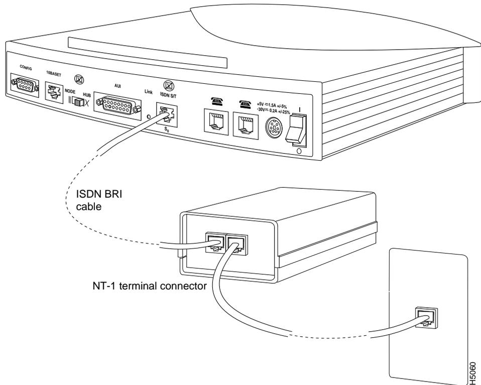
Figure 3-5 ISDN BRI Cable to ISDN BRI Wall Jack Connection (Cisco 766 Shown)
