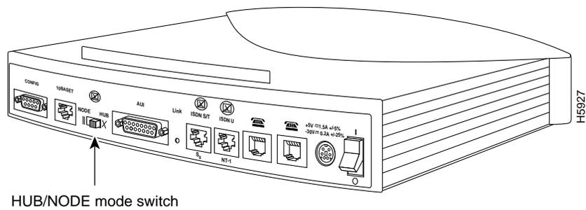
Figure 3-2 10BaseT to Ethernet Concentrator Connection (Cisco 766 Shown)
