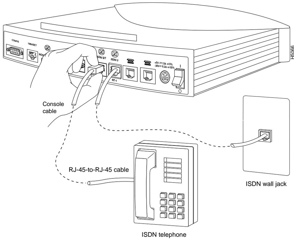
**Note** An ISDN telephone that is not self-powered requires an external power supply. Refer to the following section “Connecting an ISDN Telephone and External Power Supply” for instructions on how to connect an ISDN telephone that uses an external power supply.
