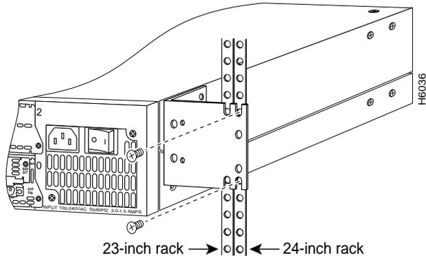
Note: The second bracket attaches to the rack at the other side of the chassis. The brackets can also be installed with the front panel forward.
