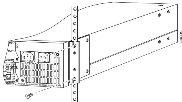
**Note:** The second bracket attaches to the rack at the other side of the chassis. The brackets can also be installed with the front panel forward.
