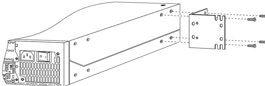
Note: The second bracket attaches to the other side of the chassis.
