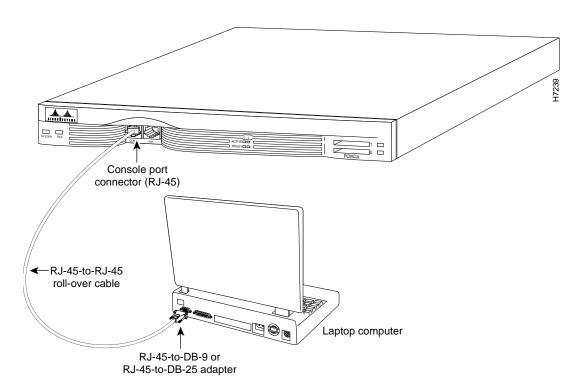
Configure your terminal or terminal emulation software for 9600 baud (the Step 2 default), 8 data bits, no parity, and 2 stop bits.
