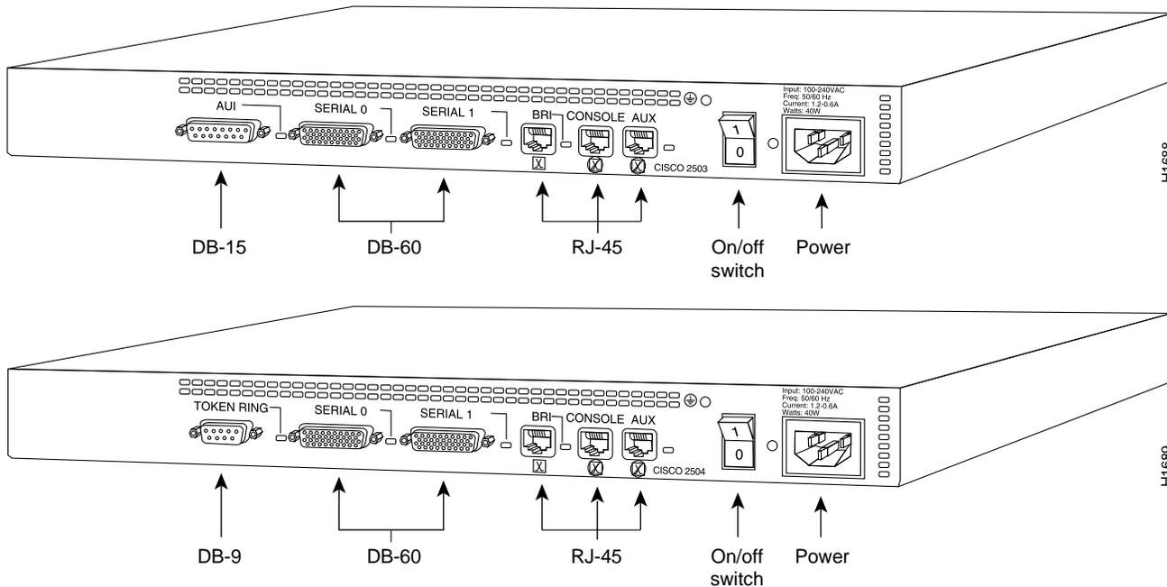
On the hub models, Ethernet RJ-45, BRI, synchronous serial, console, and auxiliary (AUX) connections are located to the left of the power connector and switch. The interface configuration depends on the model.
