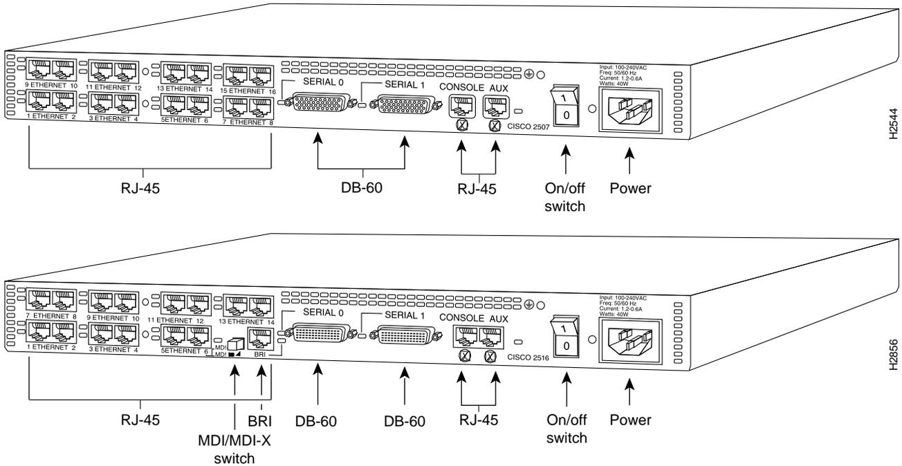
On the access server models, the ports for the Ethernet, Token Ring, asynchronous serial, synchronous serial, console, and auxiliary (AUX) connections are located to the left of the power connector and switch. The interface configuration depends on the model.
