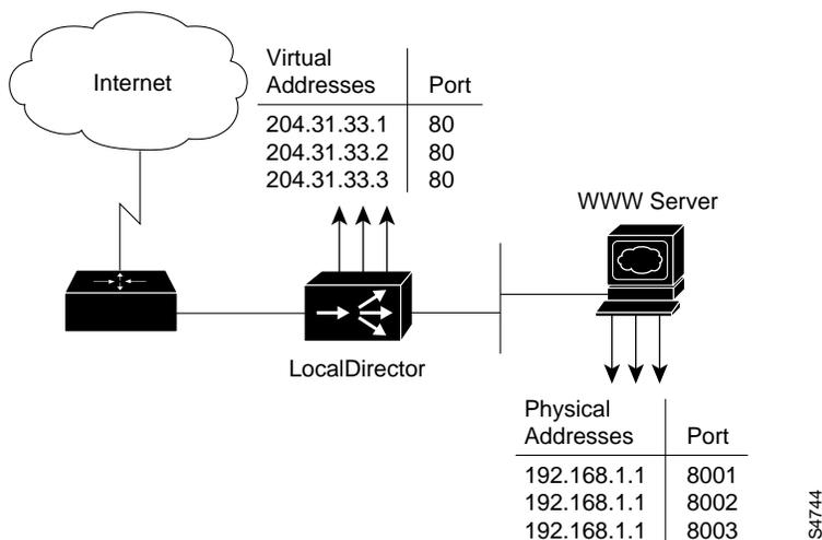
In this example, a single server (192.168.1.1) runs multiple Web server processes, each residing on a different TCP port. The outside world, however, sees the virtual addresses for three separate servers.
