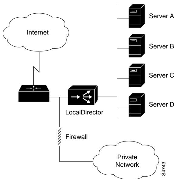
LocalDirector supports multiple IMM groups. Each IMM group consists of a virtual address multiplexed to many real servers each with a real IP address. LocalDirector measures the load on the servers specified in the IMM groups and intelligently distributes the load among those servers. In this way, LocalDirector provides nearly linear scalability.
